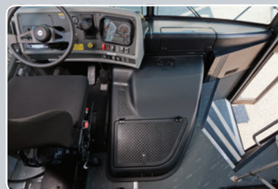
Engine access provides wider aisle for passenger loading and tool free access for serviceability.
