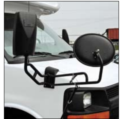
Front 6.5" x 9" flat & 6.5" x 4" convex mirrors with left and right cross-view mirrors
