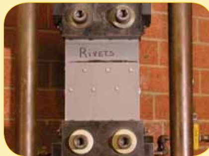
A RIVETS BEFORE: Rivets before pull test. Adhesive line showing.
