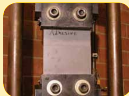
C ADHESIVE BEFORE: Adhesive before pull test.
